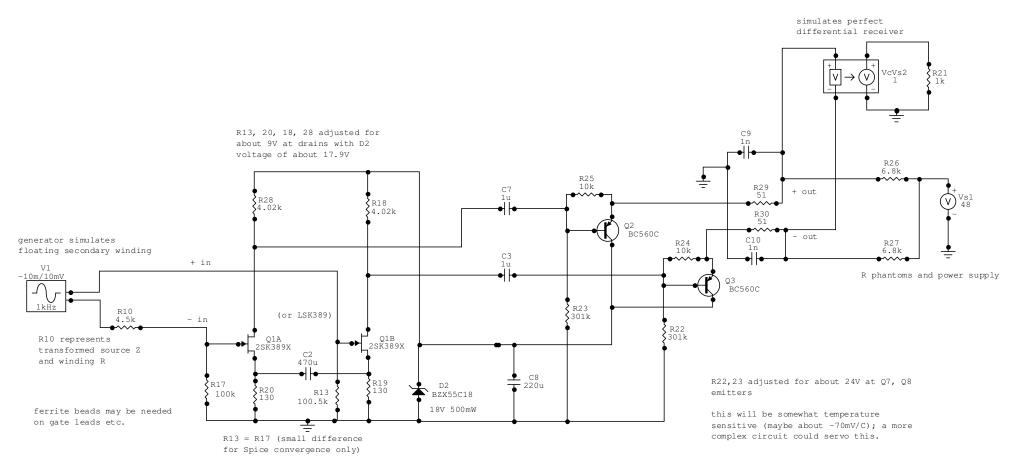
differential input C is about 180 p due to Cgd and Miller effects, plus Cgs; with the assumed source Z this means  $-3\,\mathrm{dB}$  at input is about  $190\,\mathrm{kHz}$
