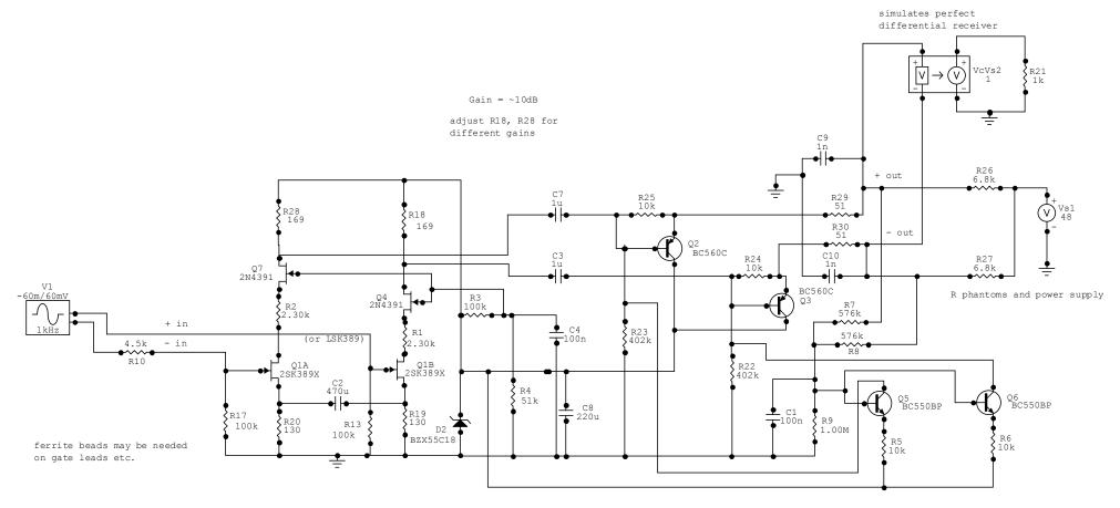
R1, R2 adjusted for small signal-induced dissipation shift; they may be eliminated for larger input signal range
